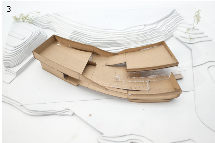
The legs of the A-shaped path merges into one, following the curvature of the hill behind. Platforms on both ends are lifted, leaving extra space for two larger amphitheatres to 'dive down' and 'look into' the boats.
