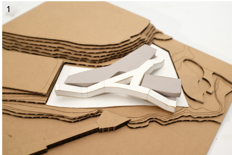
Initial study of the boathouse began with the analysis of circulation on site. The A-shaped path, hugged by adjacent mass, encourages people to converge at the center to encourage interaction.
