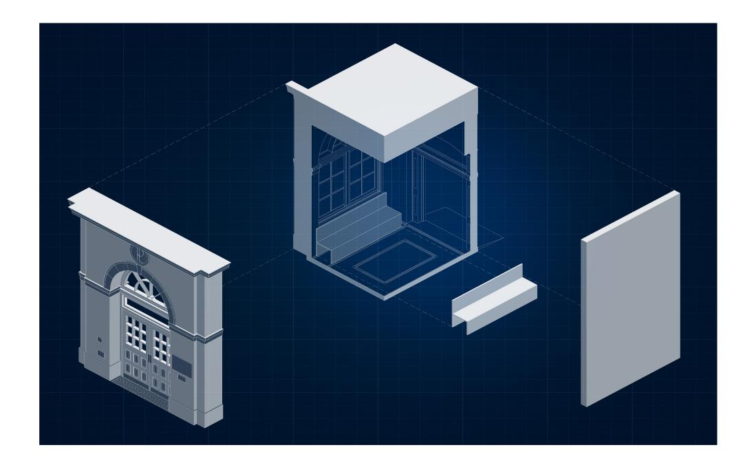
Exploded Axonometric projection created using SketchUp and Photoshop to recreate the original space with a proposed bench.
