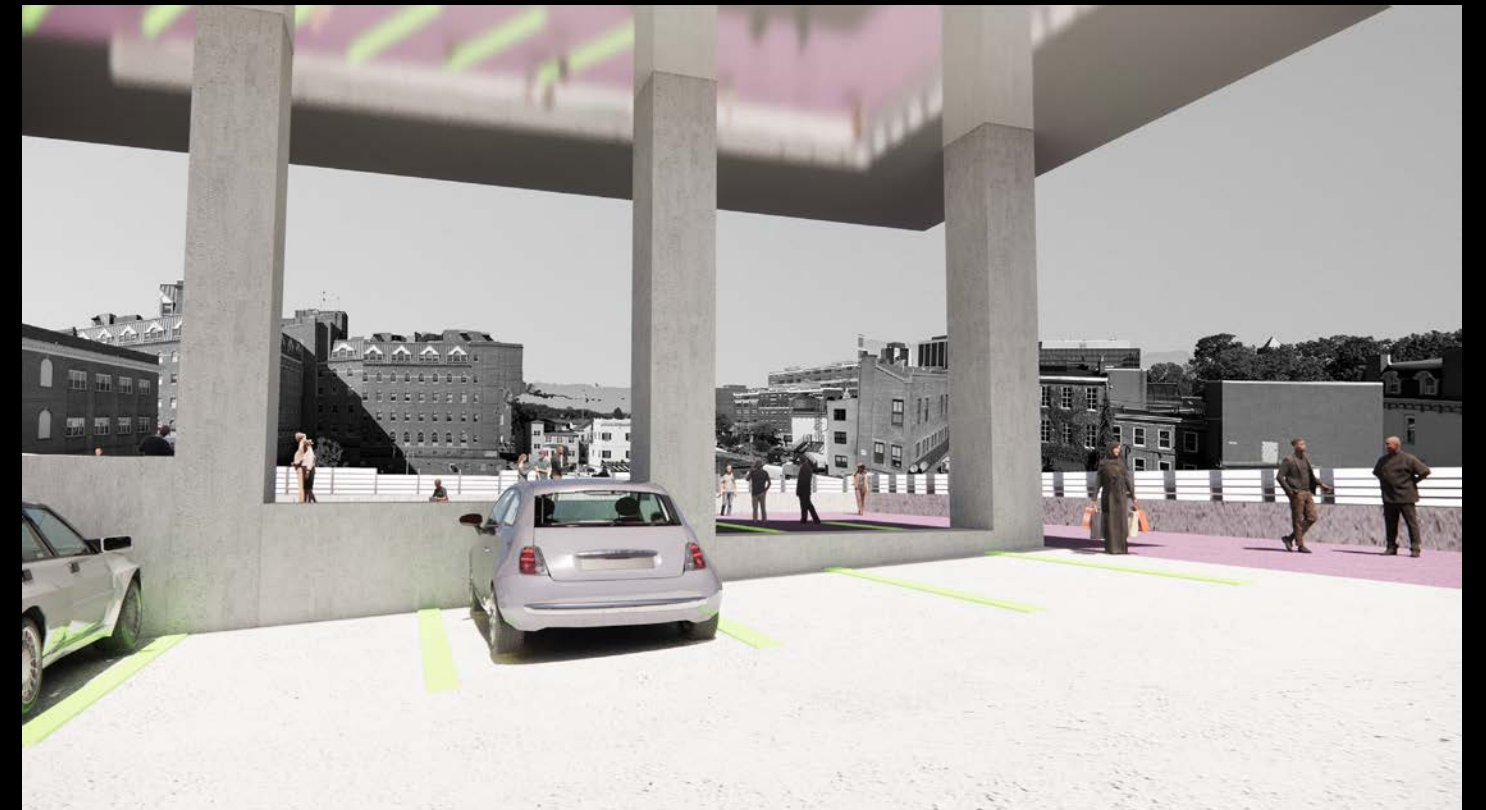
The cars are allowed to park up to where the concrete stops. The transition to no cars is by a soft boundary, that of a purple granulated rubber. The parking spots on the roof are embedded with LED strips to provide light and maintaining the gridded structure it provides the expansive observation deck.
