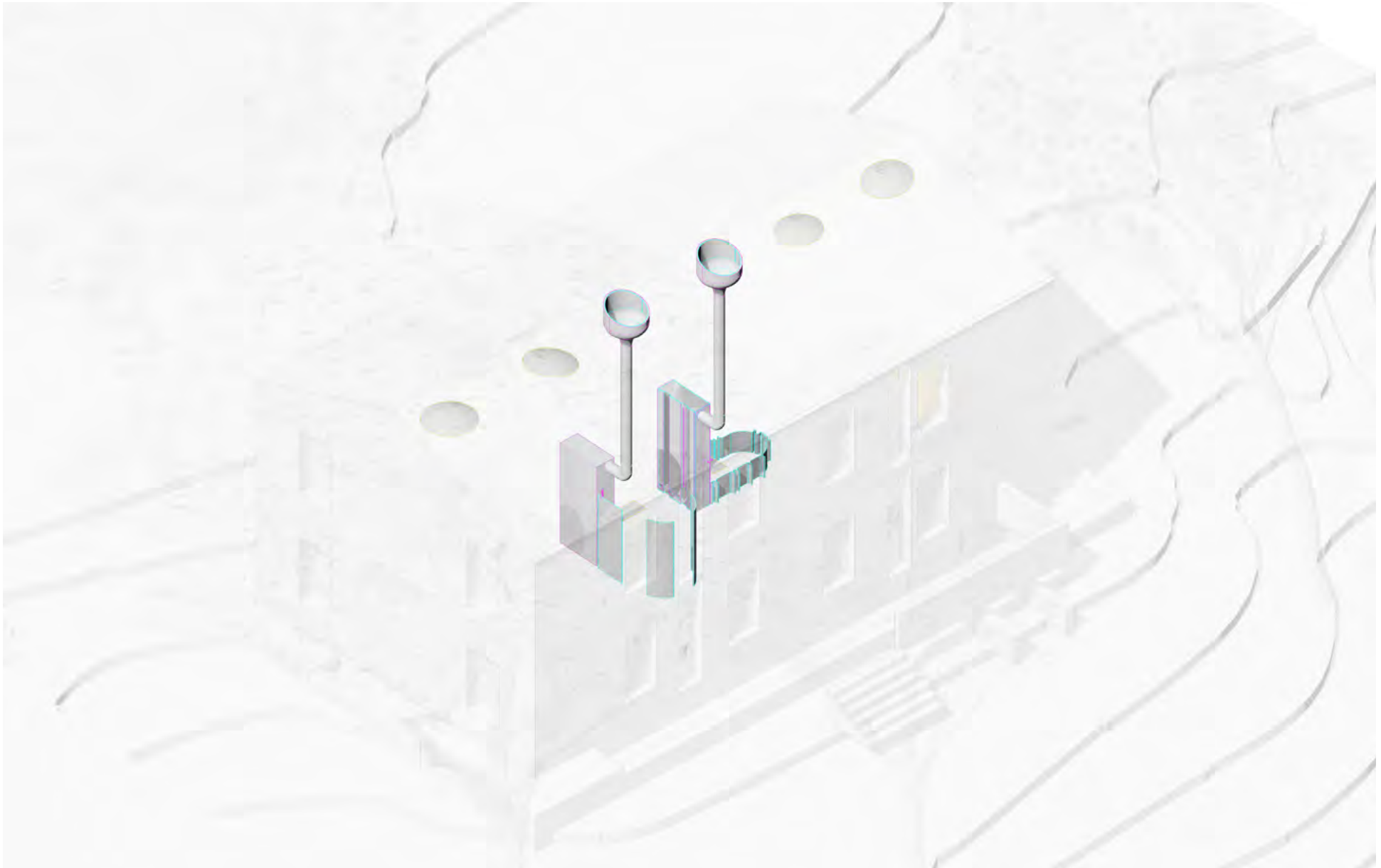
Figure 65: Light Shafts Installed within the Green Core
