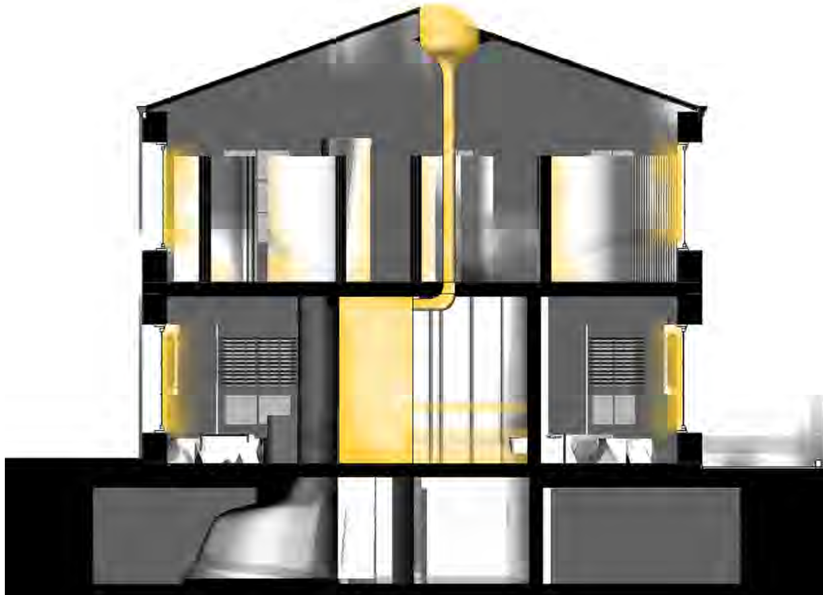
Figure 66: Building Section Explaining The Reflection Within Light Shaft And Openings Created As Per The Lux Requirement Of The Space
