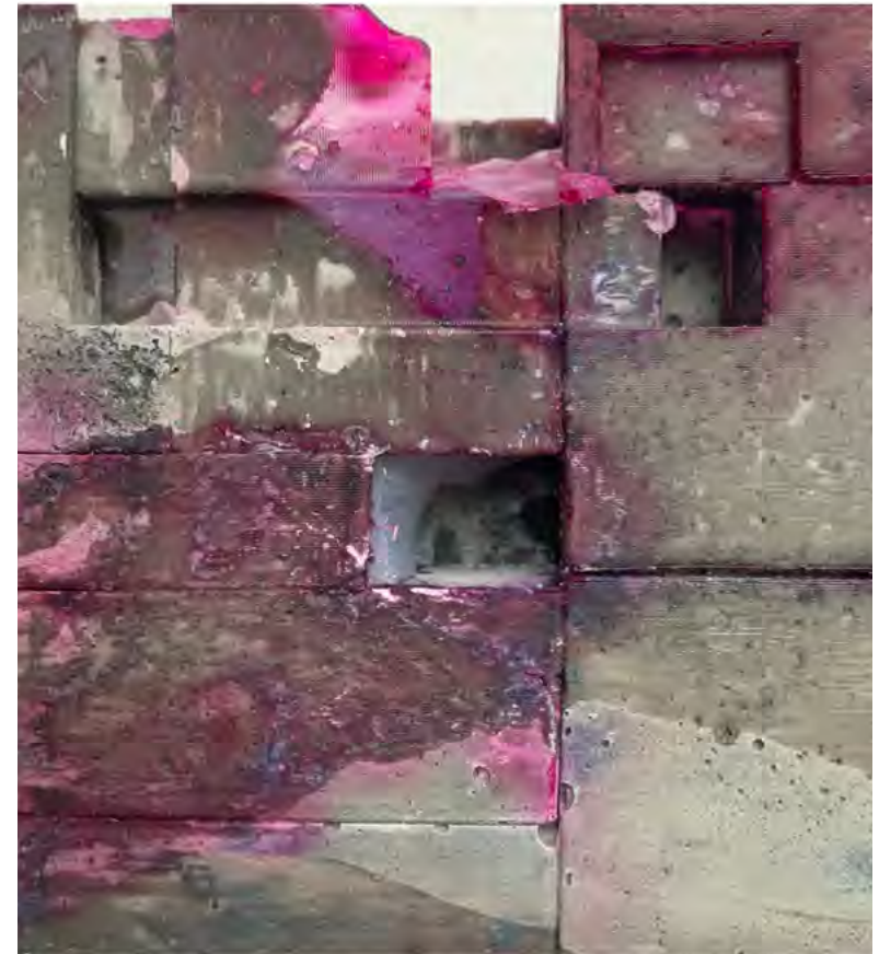
Figure 16: Casted Chunk Model in a Rockite-Resin-Pigment Recipe
