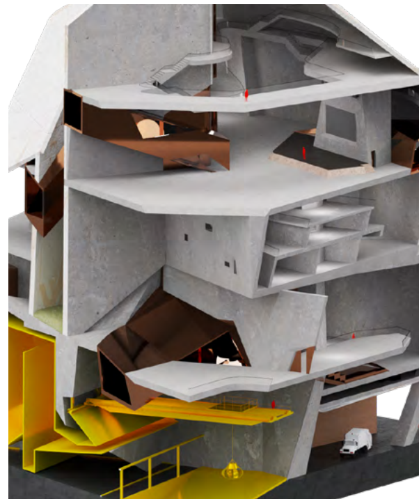
The chunk model shows the placement of the two materials on the exterior, as well as how the interior structures, sculptural columns, and floor plates interact with the metal circulation volume.
